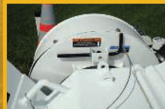
Rotor-lock pin increases operator safety
