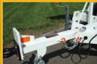
Telescopic tongue with height-adjustable pintle ring
