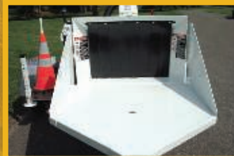
Heavy-duty folding feed table with rear jack stand and coneholder
